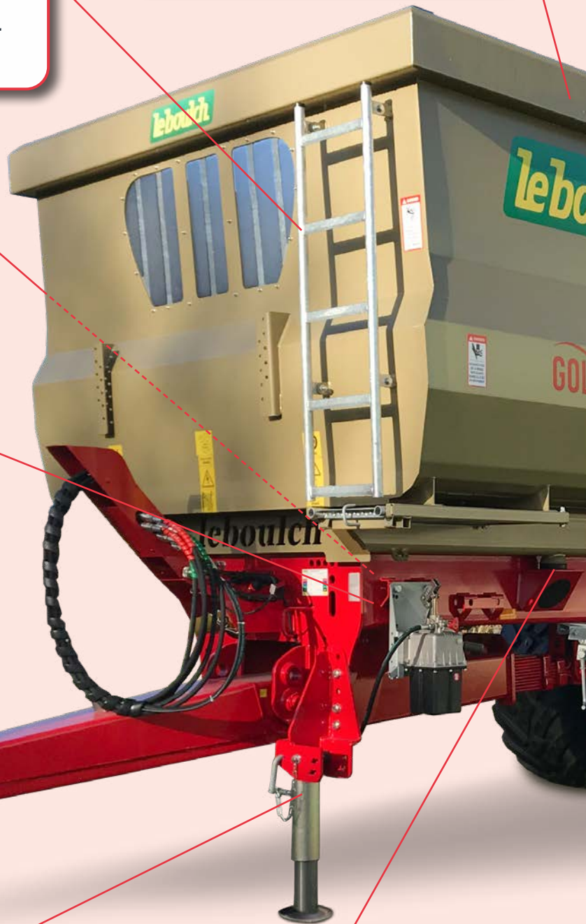
Folding aluminium ladder, galvanised side mudguards and predispositions for optional equipment (side bumper and thermoplastic mudguards).
