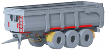
Folding aluminium ladder, galvanised side mudguards and predispositions for optional equipment (side bumper and thermoplastic mudguards).
